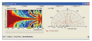
At 3 kHz a very strong side lobes are evident though the main beam is still well defined, this can present many practical problems, not least when working in reverberant spaces.
