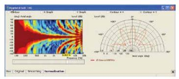
As low as 6 kHz multiple side lobes appear, effective beam control has now collapsed.
