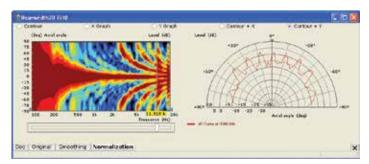
At 12 kHz the directivity characteristics are actually wider than that of a conventional loudspeaker.
