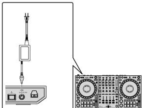
6 Press the [ $\bigcirc$ ] switch on this unit's rear panel to turn the unit on.
