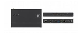
TP-590RXR is a high-performance, extended-reach HDBaseT 2.0 receiver for 4K60Hz (4:2:0) HDMI, USB, Ethernet, RS-232, IR and stereo audio signals over twisted pair. It extends video signals to up to 100m (330ft) over CAT copper cables at up to 4K@60Hz (4:2:0) 24bpp video resolution and provides even further reach for lower HD video resolutions
