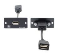
WU-AA is a single insert wall plate with one USB connector (type-A) at the front and a cable with a USB connector (type-A) connector at the rear
