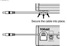
2 Connect the plug of the connection cable to the **[DC IN]** terminal. If the cable on the left side of the cable hook is too long, tighten it moderately.
