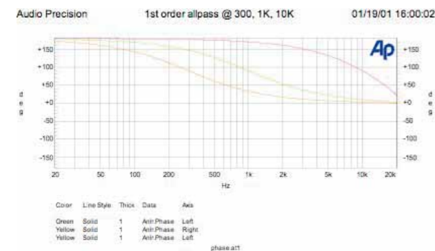
Figure 2: Response of the All Pass Filter for 1st Order phase shift at frequencies of 300Hz, 1kHz and 10kHz
