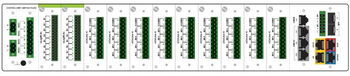
ABT-CU-11LCD/LT is a system manager combine with an audio input, audio output unit, matrix, DSP, speaker line controller and network switch in one device.
