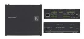
The SL-10 is a master room controller that can operate over Ethernet (LAN) with control ports that include: bidirectional one RS-485, two RS-232, three IR, two GPI/O, and five relay. It controls devices such as scalers, video displays, audio amplifiers, DVD players, sensors, screens, shades, door locks, and lights. Multiple Kramer Ethernet gateways can be used to add remote I/O ports.
