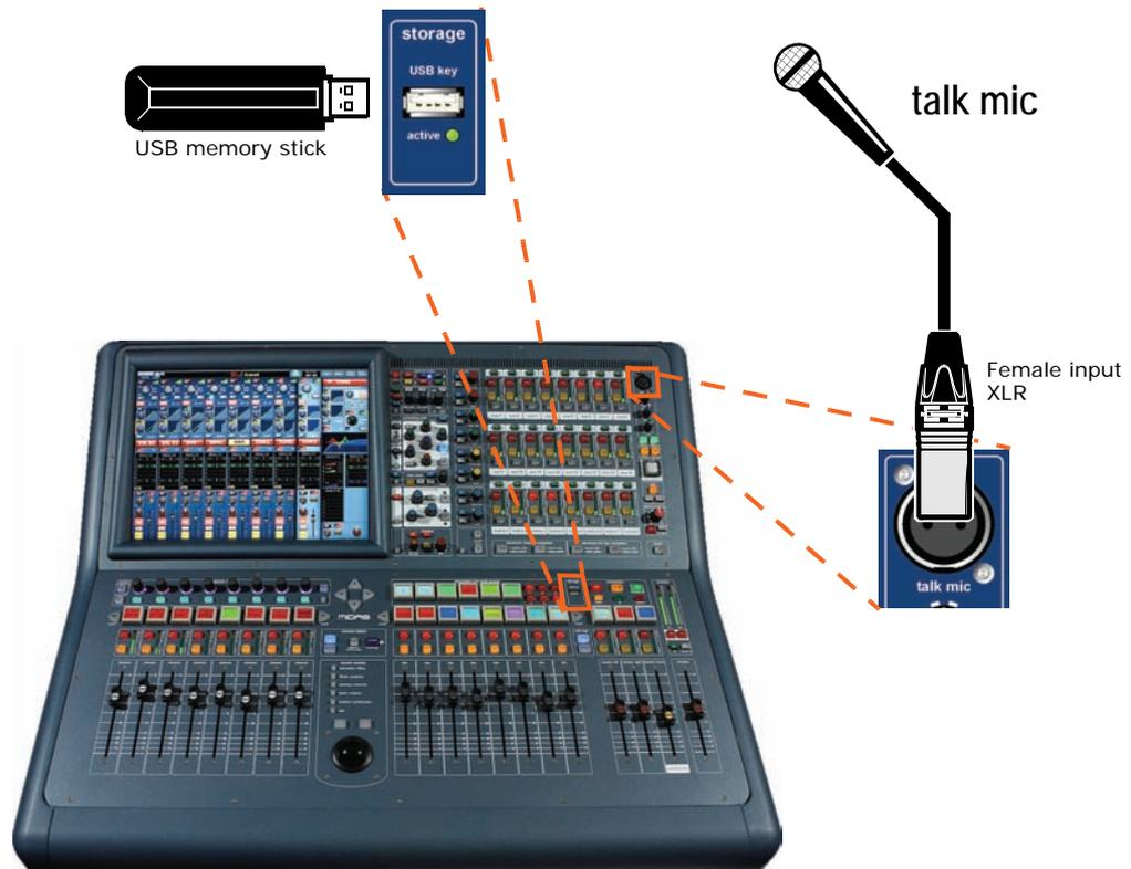
*Talk mic connector and storage USB connector on the control surface*
