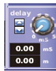
The **delay** section allows you to incorporate a time delay on an input channel, which is used mainly for mic placements and time aligning to reduce comb filtering. For example, on a drum kit mic set up, you may have a mic close to a snare drum and a couple of overhead mics. In this case, setting an input channel delay on the snare drum — to bring it more in line with the overheads — will probably produce a better sound.
