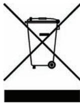
If this equipment carries a 'crossed-out wheellie bin' (shown left), please do not dispose of WEEE as unsorted municipal waste but collect and dispose of in accordance with local WEEE legislation. The horizontal bar underneath indicates that the product was placed on the EU market after 13th August 2005.
