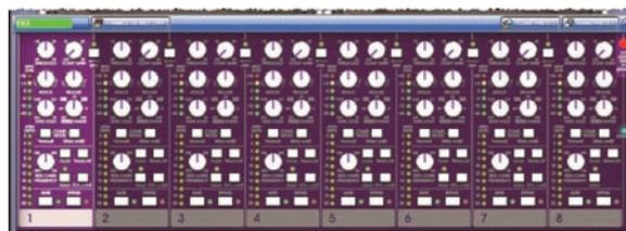
**3 Band Compressor (stereo multi-band compressor)** — is a minimum phase shift (analogue style) implementation that guarantees coherent band summing, even at the most extreme crossover point settings. Each band provides full control of its compressor's action, with partially adaptive time constants ensuring the most natural results from even the most variable sources.
