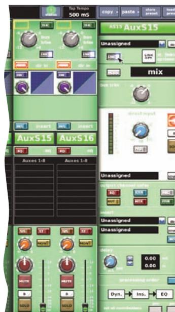
Linking is a GUI-only function, as there are no link buttons on the control surface. You can link any two adjacent input channels together. However, although each output channel has a link button only the ones on the odd numbered channels function (for example, you can link aux send channel 7 with aux send channel 8, but you cannot link aux send channel 8 with aux send channel 9).
