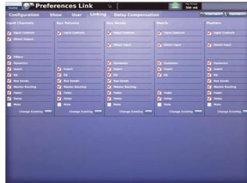
**Note:** *Deselecting a linking option (unticking its box) automatically updates the status of unlinked channels of a similar type accordingly. However, clicking **Change Existing** updates the status of all unlinked and linked channels of a similar type.*
