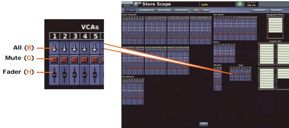
The following diagram shows the scoped parameters of the VCA group channels, and shows the **VCA Groups** screen on the GUI. This is a GUI only function.
