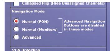
The normal (standard) modes are intended to get you up and running quickly, whereas the advanced mode enables the full power of the console control surface for the more experienced user.
