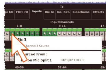
This can also be done by starting another single patch operation or by selecting another destination patch connector in the **To** section.
