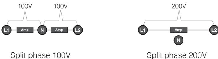
Figure 6.5: Two phase split-phase configuration
