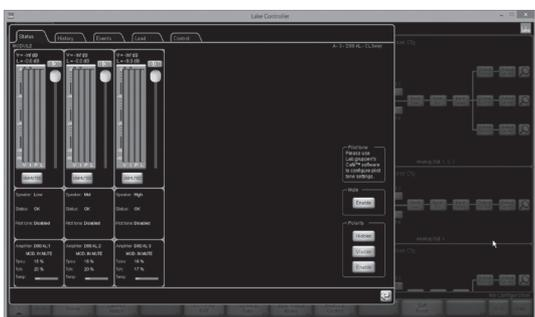
**Amplifier Events & Control, Status tab** – Drag sliders to adjust power channel attenuation and tap mute buttons to control power channel mute. Metering and Status monitoring is available for each power channel.
