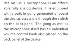
To operate the device press the MIC ON button, the status LED will switch to steady green light. In the event of an active built in gong, the status LED will turn green once the gong has ended. When finished transmitting the message release the MIC ON button to deactivate the gooseneck mic.
