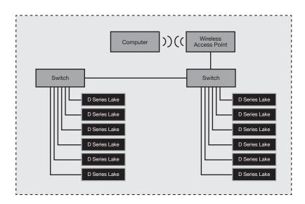
NOTE: If using Dante audio in the network, the audio traffic needs to be filtered from reaching the wireless links.
