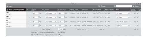
CAFÉ, RPM view - Enter power requirements and impedances for the channels to configure RPM.
