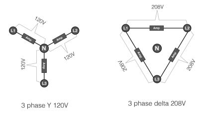
Figure 6:4: Three phase delta configuration
