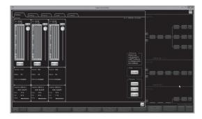
**Amplifier Events & Control, Status tab** – Drag sliders to adjust power channel attenuation and tap mute buttons to control power channel mute. Metering and Status monitoring is available for each power channel.
