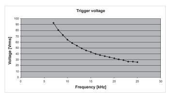
Fig 11.4: VHF Protection Frequency Sensitivity
