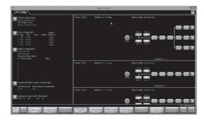
17. The right side of the I/O CONFIG screen displays a block diagram for the Modules. Tapping the different blue blocks will access the configuration screens for Input mixer, Levels, Input EQ, Delay and Output EQ/Crossover respectively. The magnifying glass at the far right end accesses the output configuration. (NOTE: Tapping the blue return button (left arrow), or the EQ/Levels EXIT button in the menu bar returns to the I/O Config screen from the various configuration screens.)
