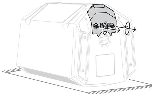
2. Gently but firmly pull on the battery pack by the finger pull located on the back of the battery door.
