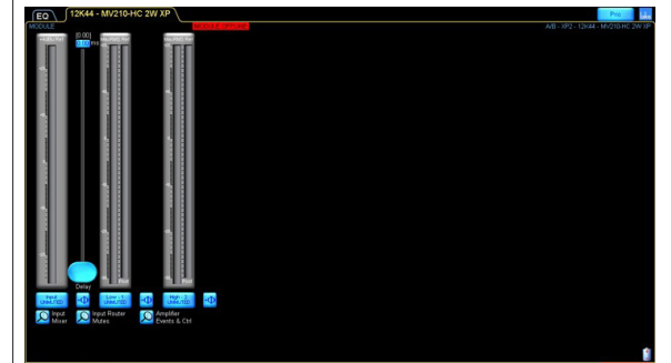
Delay adjustment of subwoofers
