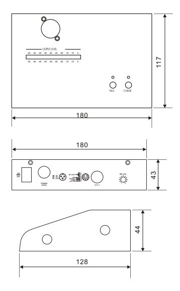
Keep the unit's all sides over 10 cm away from objects that may obstruct air flow to prevent the unit's internal temperature rise.
