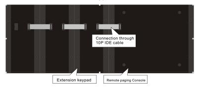
**5.3 Extension keypad dipswitch setting**: There are 4 address codes on both remote paging console and extension keypad, which are used to identify itself.
