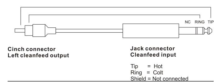
Cleanfeed output could also be an AUX send output!
